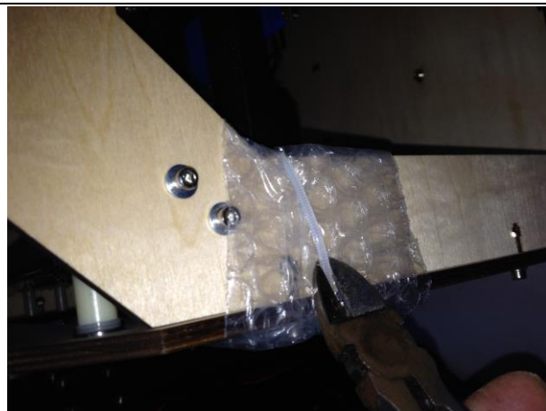
Use Water-nose pliers to cut straps fixed printhead.
