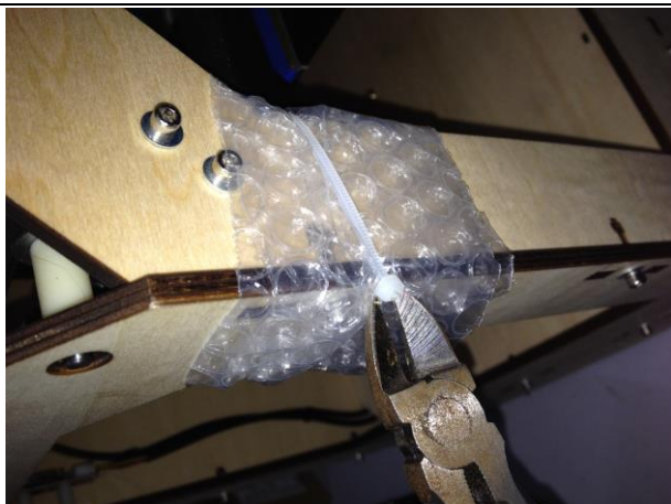
Use Water-nose pliers to cut straps fixed printhead.
